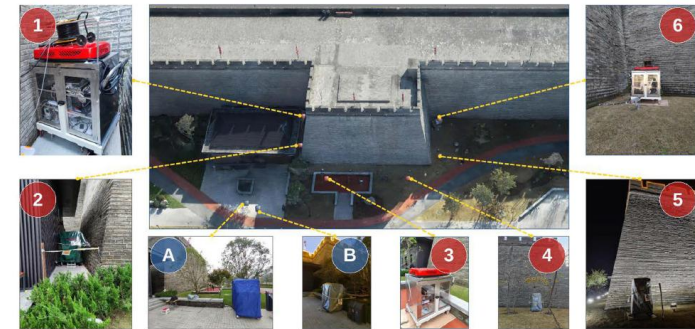
FIG. 4. Measurement location layout used in the on-site survey. Up to six detector locations (Nos. 1-6) were carefully selected with proper rotational angles facing the main body of the rampart, and two open-sky locations (a) and (b) were used to collect muon flux data without interference from any solid objects.
